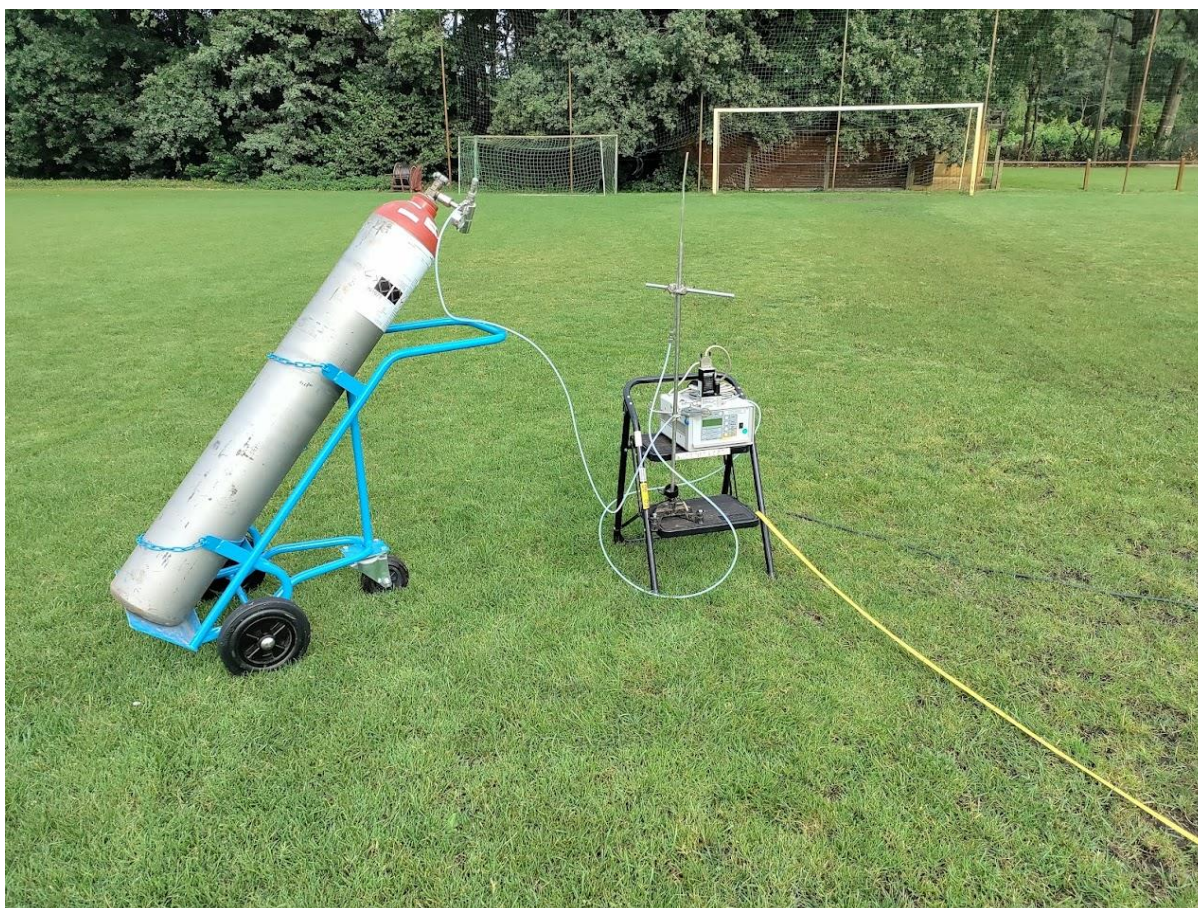
Figure 3: Picture of the methane generation unit with pure methane gasbottle and the Mass Flow Controller unit
